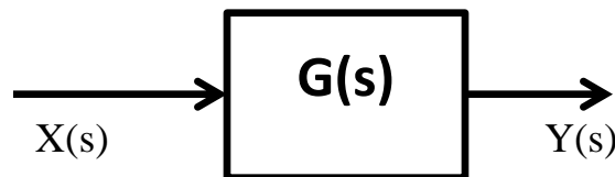
Figure 2.1 Single block diagram system
