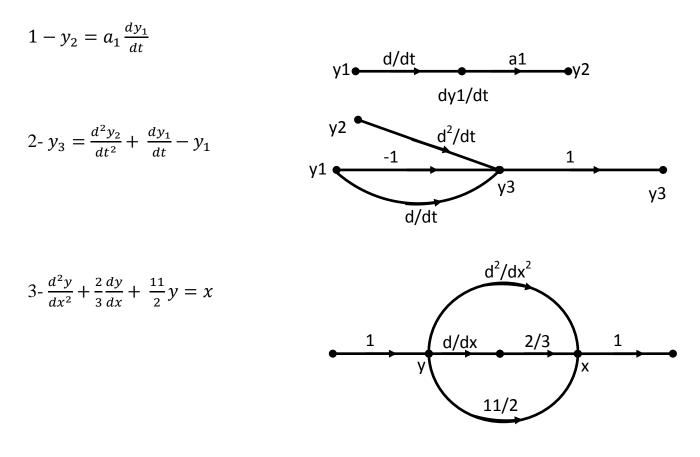
Another solution may be introduced by taking the Laplace transform of the equation as follows;
