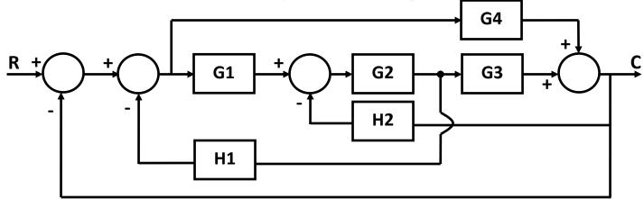
Q3- Find the transfer function for the system shown using Mason's formula.
