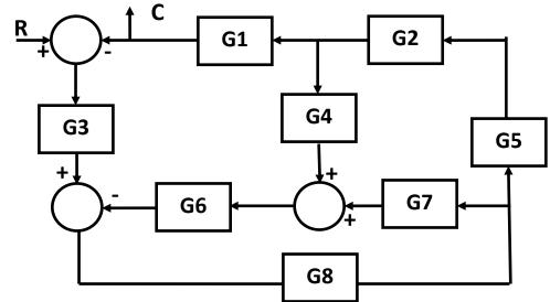
Q4- Find the transfer function for the system shown using Mason's formula.
